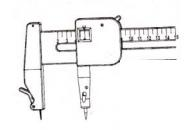
Use the Size Adjustment Knob to set the circle size – loosely tighten the knob (don't overtighten). Put the circle cutter on the paper so that both the point and the blade are touching the paper, hold the cutter straight up and down.
